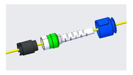
Strip cable and fit LC connector (LC connector to have no strain relief boot).
